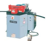
Adhering to most safety requirements it is an efficient and quicker bender used for making circular rings.
